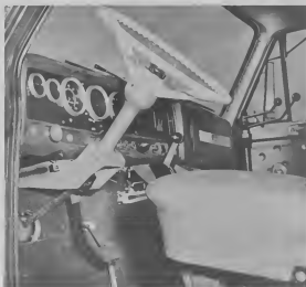
Special feature on newly acquired trucks is automatic transmission for easier driving and increased efficiency.
